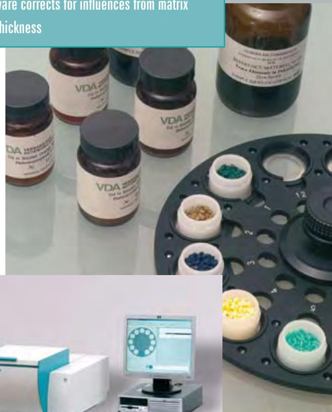
*X-ray fluorescence spectrometry is more suited to fast screening for the elements cadmium, mercury, lead, chromium and bromine than any other analytical method. It requires little or no sample preparation and is non-destructive. Even samples of polymer granulates, insulation and housing materials can be directly analyzed if necessary.*
